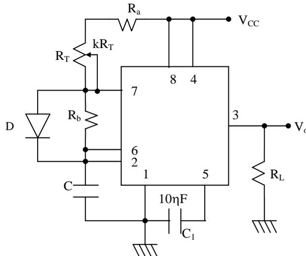
$$T_H = T_L = \left( R_A + \frac{R_T}{2} \right) C \ln \frac{2V_{CC} - 3V_\gamma}{V_{CC} - 3V_\gamma} = R_B C \ln 2 \Rightarrow R_A + \frac{R_T}{2} = \frac{\ln 2}{\ln \frac{2V_{CC} - 3V_\gamma}{V_{CC} - 3V_\gamma}} R_B$$
