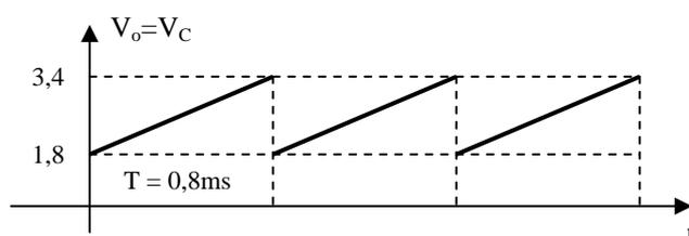
$R_1 = 270\Omega$  CH1 = 1V/div B.T. = 0,2ms/div
